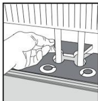
Radiator pipes, installation at radiators. Drill the holes 20 mm larger than the diameter of the pipes. Cut out the panel (with the thinnest blade possible) as per diagram. Install the plank as per normal. Glue the cut out piece back again.
