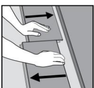
Disassembling Your floor can very easy be disassembled, which enables replacement during installation and also during use. Separate the whole row by carefully lifting up and slightly knocking just above the joint. Fold up or angle and release the whole long side. Disassemble the panels by sliding horizontally where possible or fold up and angle to release.
